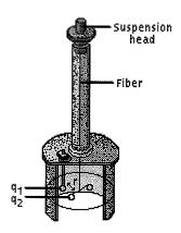
By measuring the angle of twist, Coulomb determined the force of repulsion or attraction between the charges. He also found a relation between the force, distance between the 2 charges and magnitude of the charges resulting in the following equation:
