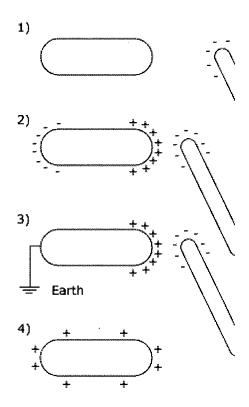
A neutral object that is connected to the Earth's surface is grounded. If a charged object is placed near a grounded object and the ground is removed while the object is still near, the neutral object becomes charged opposite to the charged object. This is called **charging by induction with a ground**. This is shown in steps 3 and 4 above. **Chargin by inductin with a ground produces oppositely charged objects**.
